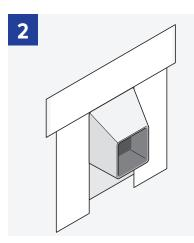
Next apply flashing over the top, shingling the side flashing.
