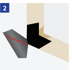
Smooth the dove-tailed edge of the Flash Corners over the sill and adhere to the vertical wall face. Make certain any bubbles or wrinkles are smoothed out.
