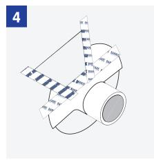
Tape over the 45° cuts using Barricade Seam Tape.
