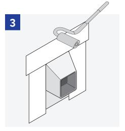
Use a roller to apply even pressure along the flashing, being sure to push out any air pockets that may have appeared. Barricade suggests finishing with Barricade Bear Caulk commercial sealant to ensure a tight seal around the edges of the penetration.
