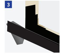
Repeat Steps 1-3 for the other corner of the window. Overlap the horizontal flanges of Barricade Flash Corners with a measured piece of Barricade Flash Ulti or Barricade Flash Extreme window flashing. Flash remaining portion of window per the building code.
