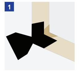
Peel back paper-release liner and discard. Adhere square-edged side of Barricade Flash Corners to a front. inside sill corner. Ensure the front edge of the material is flush with the front edge of the window opening.
