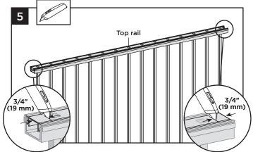
How to Measure and Cut Top Rail for Post-to-Post Configuration
