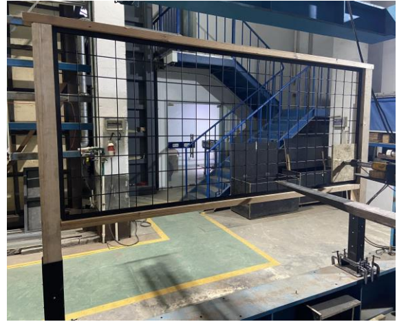
Fig 1. In-Fill Load Test at lower-right corner
