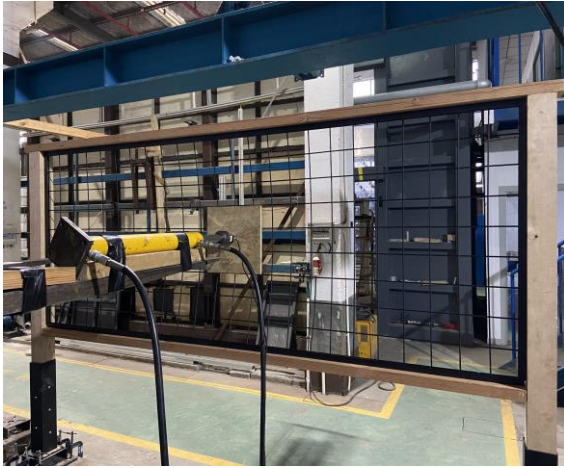
Fig 1. In-Fill Load Test at central position
