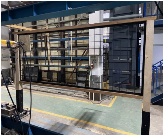
Fig 3. In-Fill Load Test at upper-left corner
