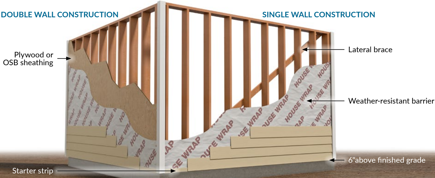
Double and Single Wall Construction
